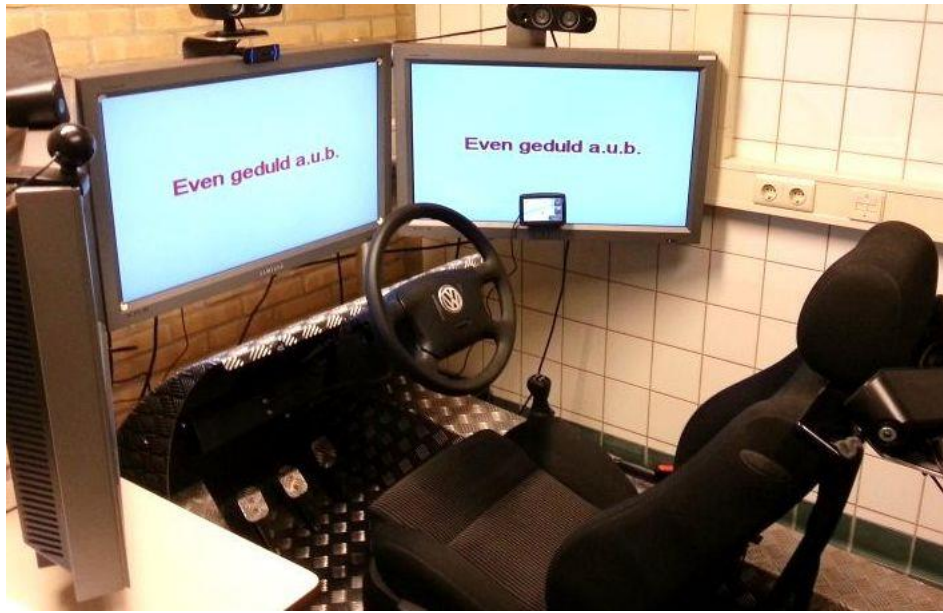
Figure 5.1: The driving simulator, with the touch screen navigation system attached to the right-hand screen.
