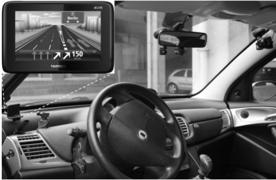
Figure 7.A1: Vehicle cabin layout (Lancia Ypsilon), including a navigation system photo. The navigation system mount is installed to the left of the steering wheel, with a camera facing it. In the Peugeot 207 the system was mounted to the right of the steering wheel.
