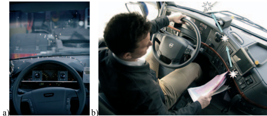
Figure 14 a) and b). Examples of a visual distraction alert that redirects gaze using flashing LEDs, a) the first implementation used strings of smaller LEDs running along the doors and centre console towards the road centre. The LEDs at road centre were reflected on the windshield. Foto: Lars Ardarve. A later version used three strong LEDs as illustrated in b) with the last LED reflecting on the windshield. Foto: Volvo Truck Corp.
