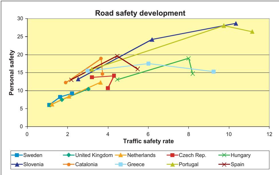
Figure 2.6. Development of road safety in SUNflower+6 countries, visualized as personal safety (fatalities per 100 000 inhabitants) versus the traffic safety rate (fatalities per 10 000 vehicles). Time development from the 1981-1983 period for points at the right side of the graph, via 1991-1993 to 2001-2003 for points at the left side of the graph.
