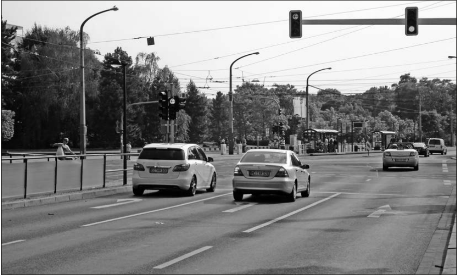
Figure 60: Example of a protected left-turn regulation with separate green phases for turning left versus going straight (source: SaMERU, 2013).
