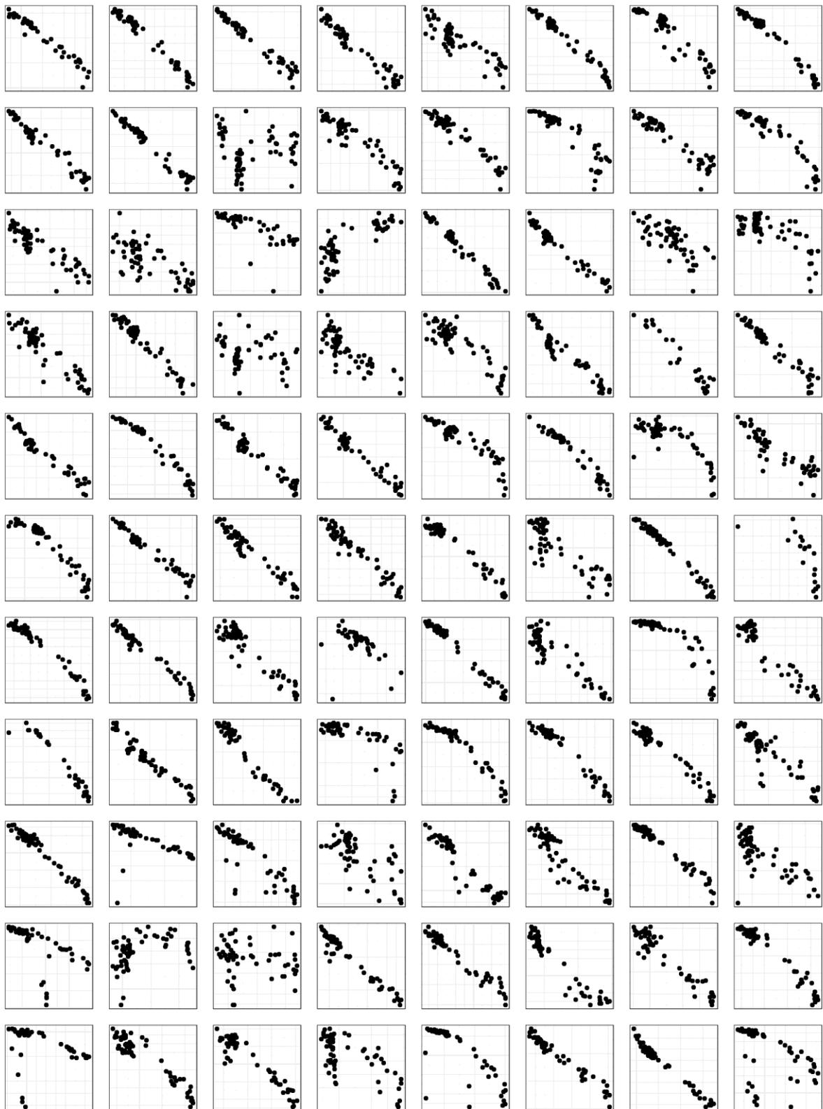
FIGURE 15 – SCATTER PLOTS FOR INDIVIDUAL SITES COMPARING LOG(% OVER LIMIT +15MPH) TO TOTAL DAILY FLOW
