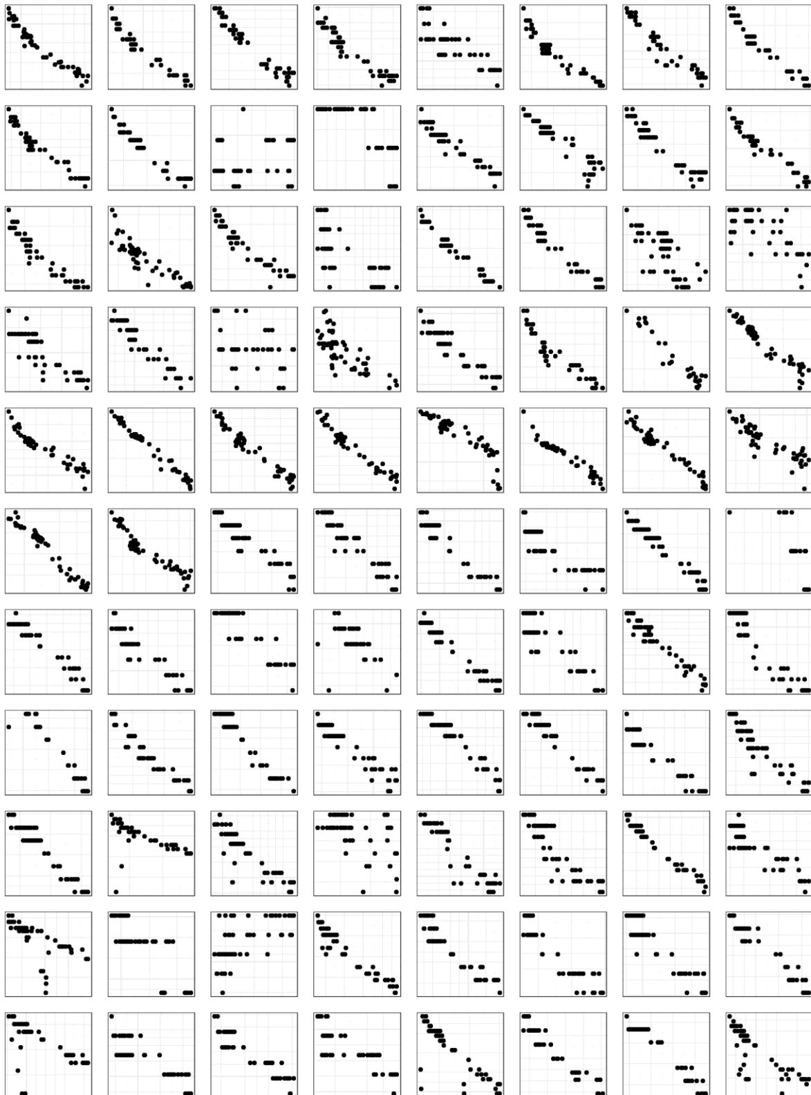
FIGURE 14 – SCATTER PLOTS FOR INDIVIDUAL SITES COMPARING LOG(% OVER LIMIT) TO TOTAL DAILY FLOW
