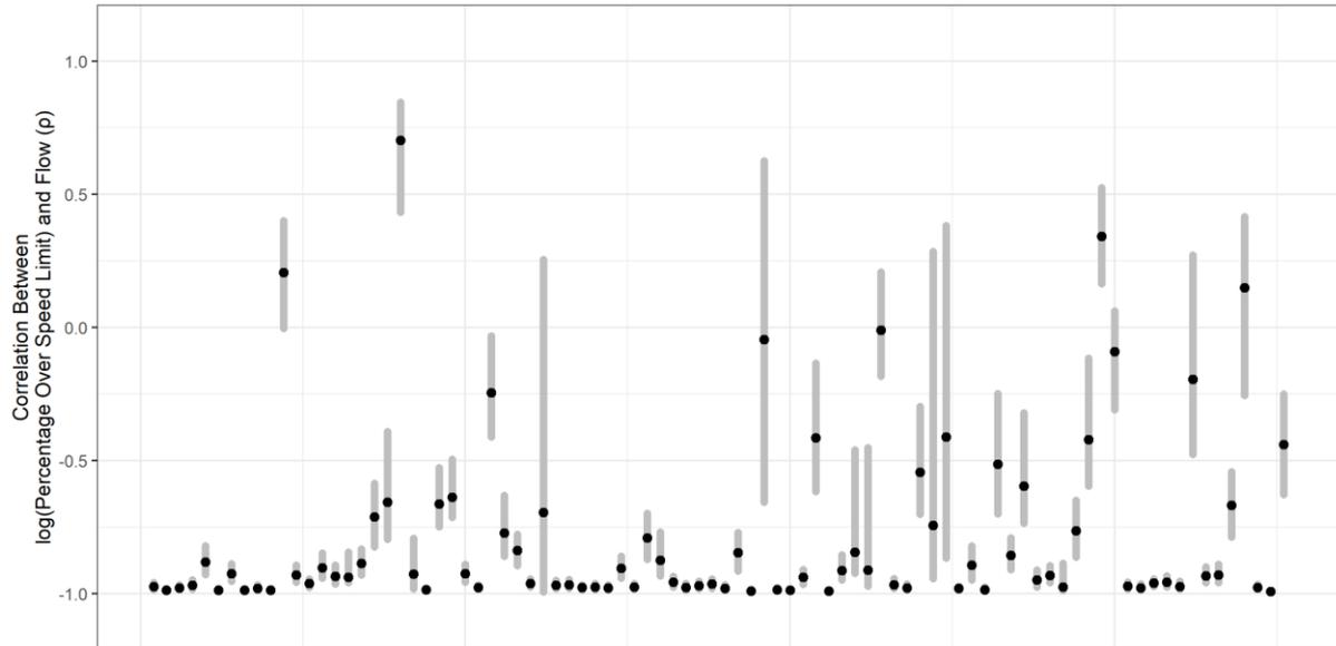
FIGURE 10 – CORRELATION VALUES BY SITE COMPARING LOG(% OVER LIMIT +15MPH) TO TOTAL DAILY FLOW
