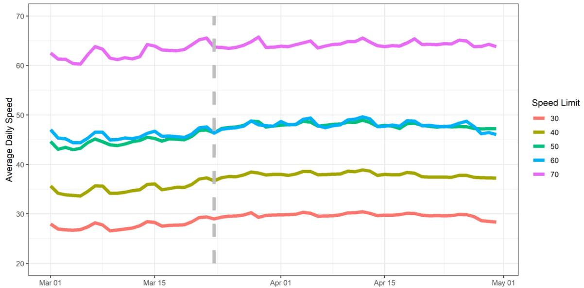
**FIGURE 3 – OBSERVED CHANGES IN AVERAGE 85<sup>TH</sup> PERCENTILE SPEEDS BEFORE AND AFTER THE LOCKDOWN**
