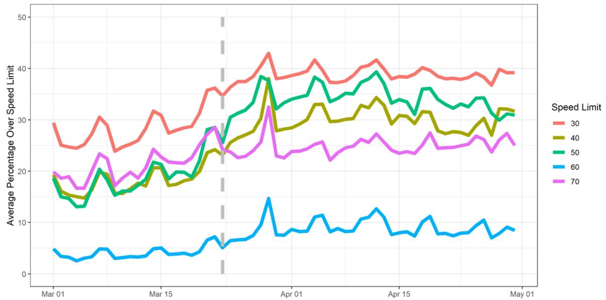
**FIGURE 5 – OBSERVED CHANGES IN THE AVERAGE PERCENTAGE OF VEHICLES MORE THAN 15MPH OVER THE LIMIT BEFORE AND AFTER THE LOCKDOWN**
